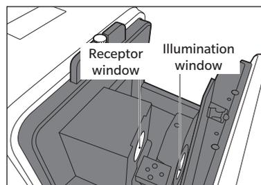
**3 Close the transmittance specimen chamber cover.**
