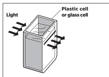
**3 Close the transmittance specimen chamber cover.**
