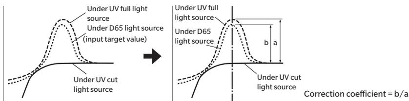
The fluorescence correction coefficient is used to determine the fluorescence reflectance through numerical processing of a measurement object's reflectance under the UV full light source and under the UV cut light source. (The reflectance of the cut wavelength region for UV cut lighting is uniform at 0%.)
